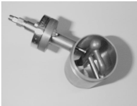
Figure 8: Cu model of the HOM coupler for the Nb-prototype of the superstructure. This coupler is based on the 40 mm TTF HOM coupler for the 9-cell cavities. The length of the tip is increased by 5 mm to fulfil the requirements on damping.
