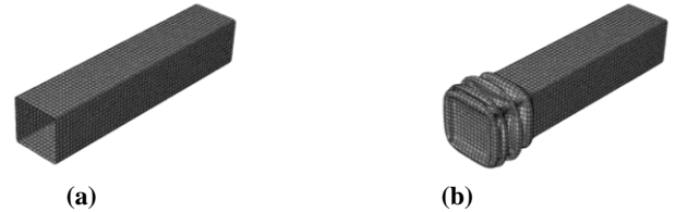
FIGURE 4: DEFORMATION AFTER 5MS OF INITIAL IMPACT (A) DEFORMATION OF COMPOSITE RAIL; (B) DEFORMATION OF ALUMINUM RAIL
