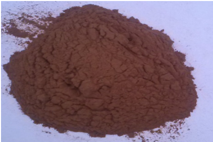
Plate 2. 80 \mu\text{m} Coconut shell Powder
