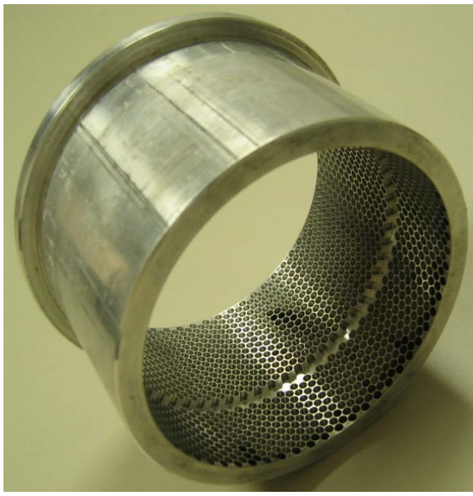
Figure 3 Seal with groove
