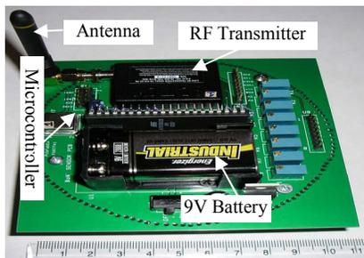
Figure 6. The printed circuit board incorporating the RF transmitter and microcontroller. A 9 V battery supplies power to the board. A 5 V voltage regulator drives the electronics. The board consumes around 27 mA at 5 V (135 mW) and measures 10.2 cm × 10.2 cm. The RF module can deliver up to 1 mW of output power.
