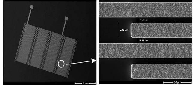
Figure 7. SEM images of the fabricated microcapacitor. (a) The entire microcapacitor. (b) The interdigitated microcapacitor electrodes. The electrodes have a width of about 9.4  $\mu\text{m}$  separated by a gap of about 3.5  $\mu\text{m}$ .
