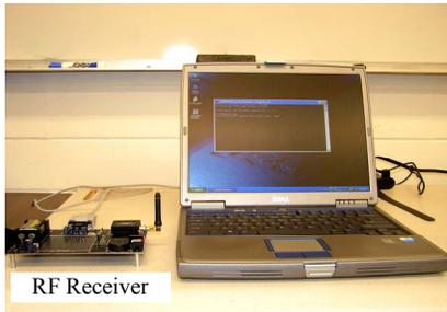
Figure 5. The wireless receiver. The RF receiver is interfaced to the serial port of the computer through the RS-232C standard. The computer employs a 'C' program to determine the time difference of the two received sensor signals.
