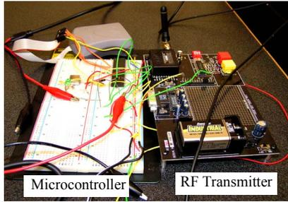
Figure 4. The wireless transmitter using a bread-board based design. The microcontroller and RF transmitter form the wireless transmitter operating at 916.48 MHz and 9600 baud with a bit error rate less than  $10^{-5}$ . The range of transmission is about 150 ft inside a concrete building.
