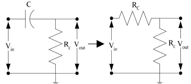
Figure 8. The transduction circuit. The microcapacitor with interdigitated electrodes is connected to an external resistor to form a high pass RC circuit. Upon dissolution of the membrane, the slightly conductive target species enters the microcapacitor and transforms it into a resistor. Thus, an output voltage results following membrane dissolution. This voltage is sufficient to drive the input ports of a microcontroller directly.
