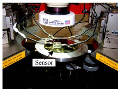
Figure 3. On-wafer testing is accomplished using a Karl Suss PM5 probe station. Probes are used to connect the output of the sensors to the microcontroller.
