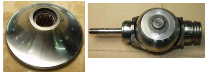
Figure 16 - Traction Drive Elements after Endurance Test
