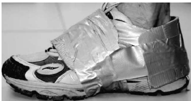
FIGURE 1—Subject with 4-kg load attached to the foot. Lead strips were wrapped around the heel and over the dorsal aspect of the foot and secured with duct tape.
