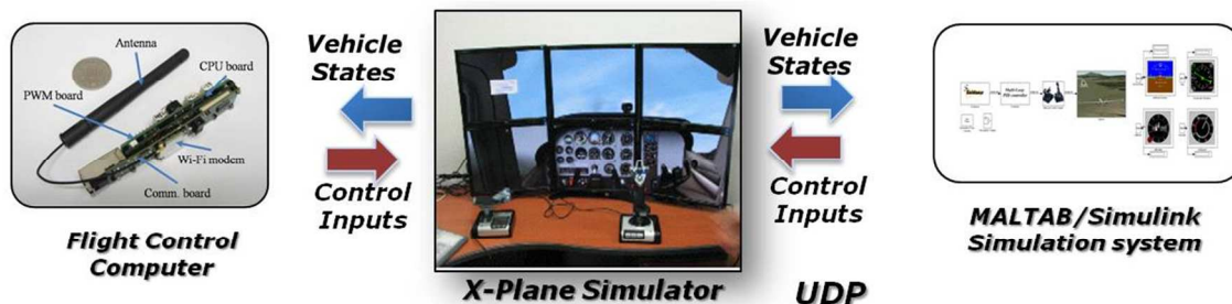
Figure 24. MATLAB/Simulink based PILS system using X-Plane
