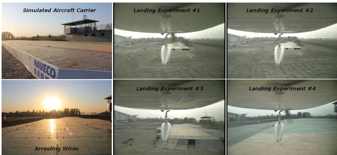
Figure 30. Automatic takeoff and landing experiment on simulated aircraft carrier (a simulated carrier(left), landing scenes from onboard video (right))
