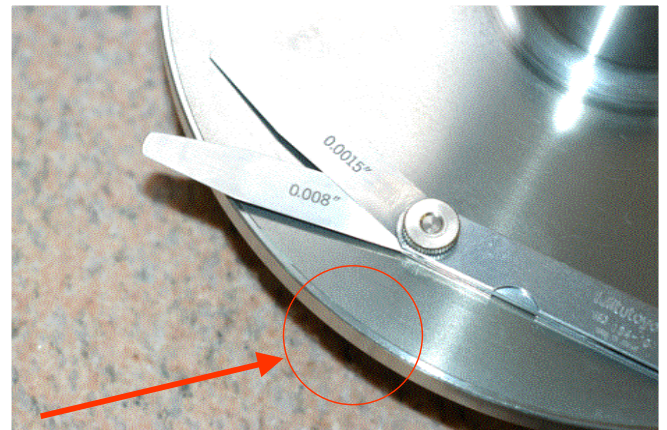
Figure 11. Coating instability showing shrinkage at the rim.
