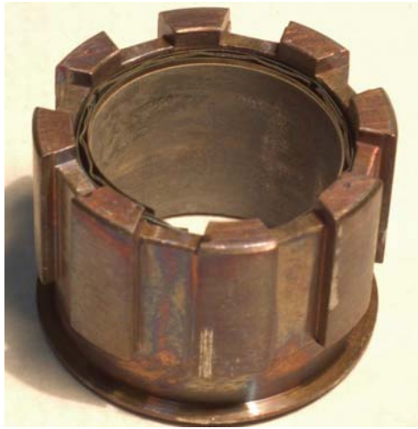
Figure 9. Nickel-chrome based coated foil bearing after 850°C test in oil-free turbojet engine.
