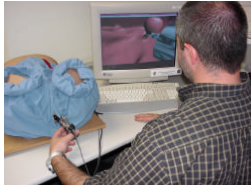
Figure 9. To grasp a polyp, an endoscopist manipulates the handle on the plastic pelvis model, which hides the haptic feedback hardware.
