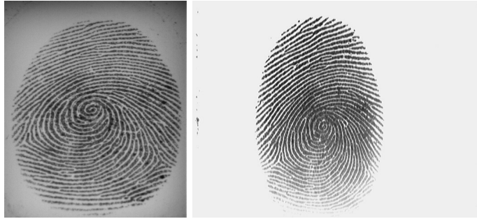
Figure 1: Example of same fingerprint from Biometrika FX2000 (left), Italdata ET10 (right) scanner.
