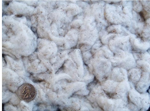
Figure 4. Photograph of typical trash captured by the battery condenser system cyclones.
