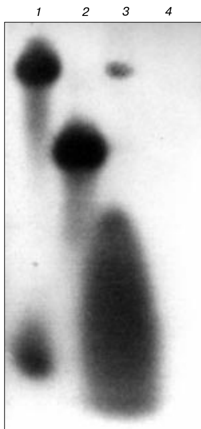
Fig. 1. Autoradiogram of electrophoretically analyzed transcripts (20% polyacrylamide gel, 7 M urea): 1) heterologous 32 P-labeled 20-base oligoribonucleotide (upper band) and [α- 32 P]CTP; 2) heterologous 32 P-labeled 9-base oligoribonucleotide; 3) transcript; 4) transcription in the presence of α-amanitin.
