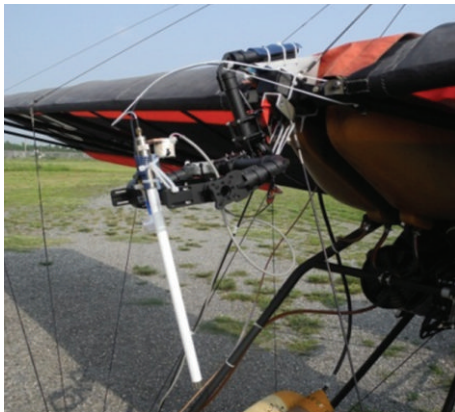
FIGURE 12: Airborne antenna on JJ2071 for ULAFP test.
