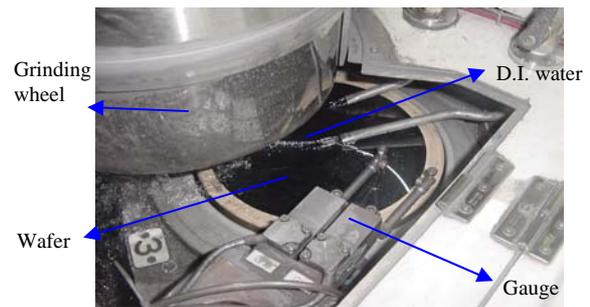
Fig. 3. Photo of grinding arrangement [3].
