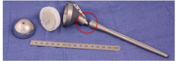
Figure 1 | The retrieved TSR, in which fracture occurred at the metaphyseal-diaphysis screw junction (circled).
