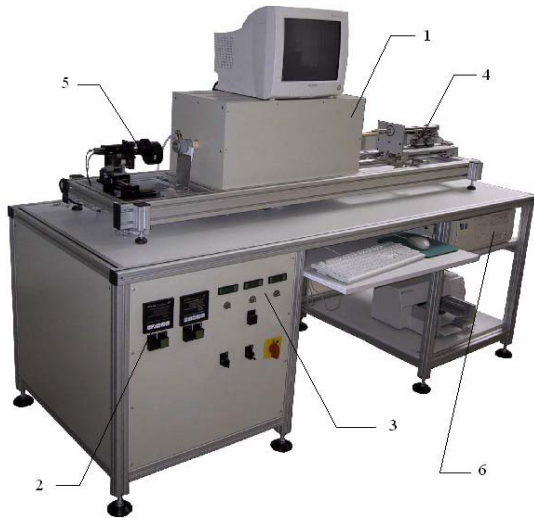
Fig.1. The general view of "Thermo-Wet" system; 1- high-temperature electric furnace; 2- system for the precise temperature measurement and control; 3 - technological gases supply system; 4- specimen insertion mechanism; 5- vision unit; 6- computer;
