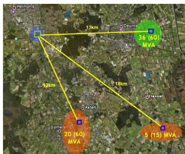
Figure 3. Areas with CHP-plants in the neighbourhood of Helmond (picture courtesy of Google Maps)
