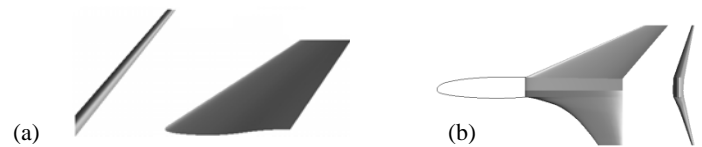
Figure 10. Winglets: (a) vortex diffuser; (b) tip fence.
