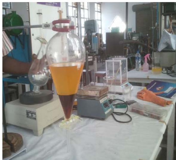
Figure-8. Alkaline transesterification: Biodiesel at top layer and Glycerol at bottom layer.
