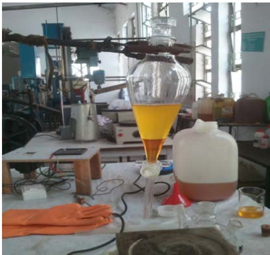
Figure-3. Acid esterification: Low FFA oil at bottom layer and excess methanol with sulphuric acid at top layer.
