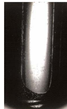
Fig. 4 Initial bubble formation stage for pure water at t = 2.40 s after decompression and for water mixed with a surfactant at t = 3.60 s after decompression. The bubble formation time in this case is t_b = 1.83 s.
