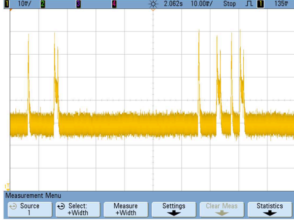
Fig. 4. Example of a trace of the voltage of the IRIS mote. The mote is set to transmit 32 bytes of payload continuously.
