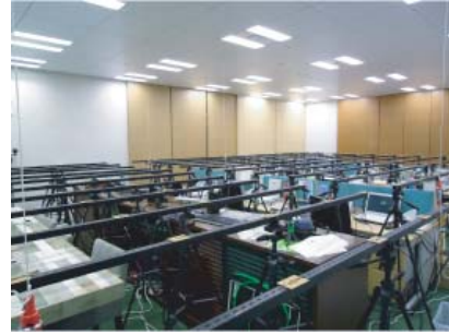
Fig. 7. Illuminance distribution measurement in Ecozzeria
