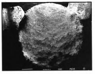
Fig. 8 — Fracture surface of the Ni-20Cr powder interlayer.
