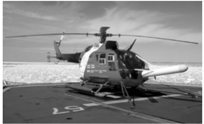
Fig. 1 "EISFlow™" Electromagnetic Induction sensor mounted on a Canadian Coast Guard B0105 helicopter onboard the CCG icebreaker Edward Cornwallis .
