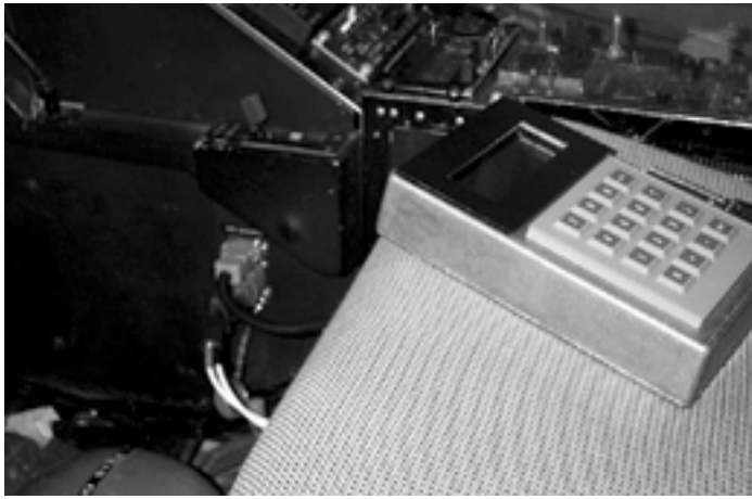
Fig. 2 The hand-held operator's control unit on the front passenger seat with power and GPS input connectors to the helicopter shown in the background.
