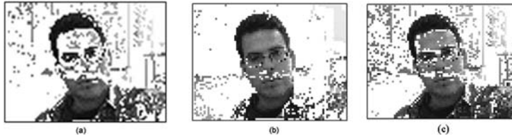
Fig. 4 Background subtraction in: a) RGB; b) HSI; and c) normalized r, g .
