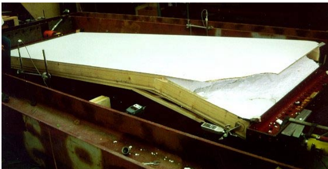
Figure 16 typical failure caused by buckling perpendicular to the plane of the panel
