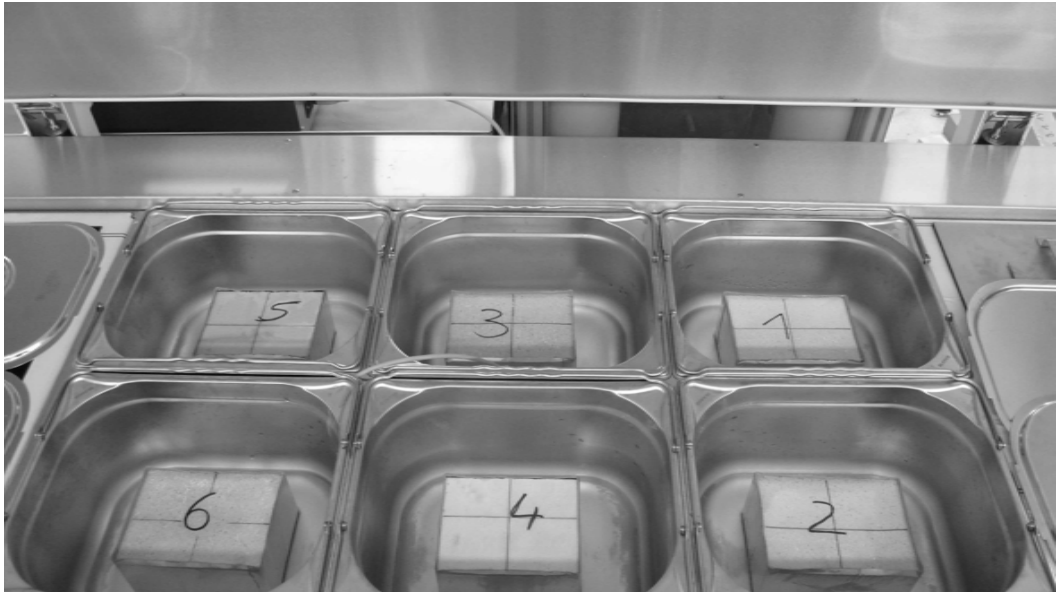
Figure 3. Determination of the Capillary Suction of De-Icing Solution and Freeze Thaw Test
