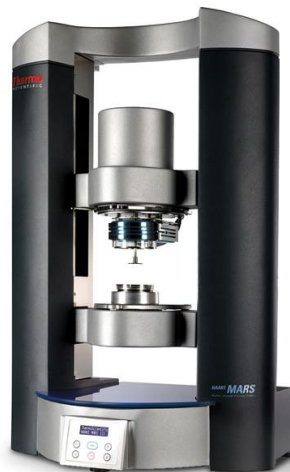
Figure 1: Rheometer HAAKE MARS For Rheological Measurements (Origin: Thermo Scientific)
