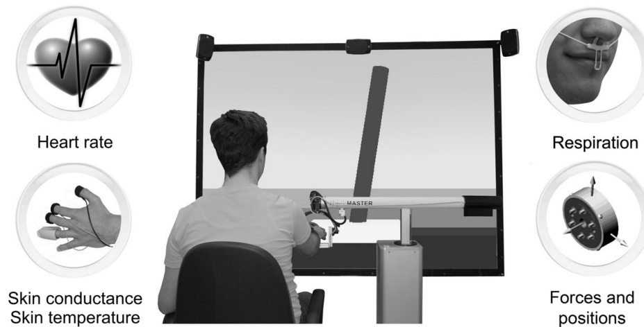
Fig. 1. The hardware configuration and virtual scenario. The subject is seated in front of a screen (centre) and manipulates the HapticMaster (1) with his/her dominant arm. The screen displays the inverted pendulum balancing task with the virtual cart (2) and pole (3). The circles on the left and right show the sensors used. The force and position sensors are integrated into the HapticMaster while the physiological sensors are attached to the subject.
