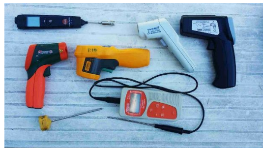
Figure 3. Contact thermometers (Bios in bottom left, Oakton Acorn in bottom right) and five IR thermometers (above), four of which are pistol-shaped.
