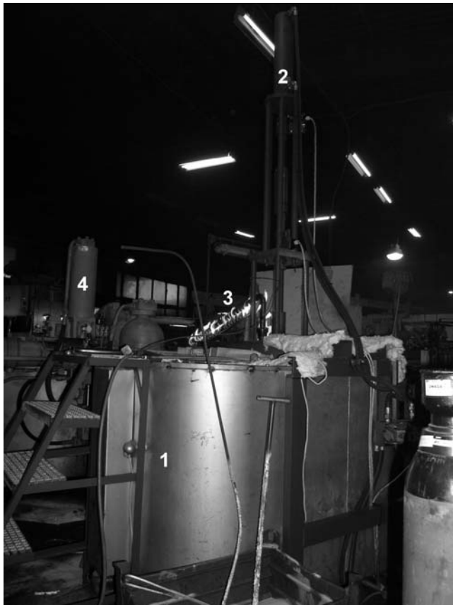
Fig. 2. Photograph of the cold-chamber die-casting line for magnesium alloys in the "SILUM" Foundry: 1 – furnace with two-chamber crucible, 2 – metering pump, 3 – transporting tube, 4 – cold chamber die-casting machine
