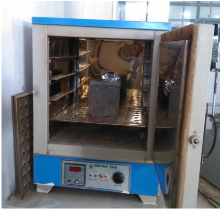
Figure 3. Cube in oven while heating
