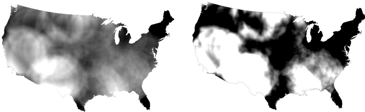
Figure 4: Histogram contrast stretching as applied to the raster model’s output. Two standard deviations (left), 0.5 standard deviation (right).
