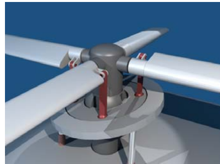
Figure 1 : Schematic of a helicopter swashplate
