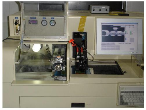
Figure 10. Photo of automatic wafer dicing
