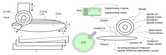
Figure 8. Working path for the dicing Figure 9. Peripheral equipments and signals in dicing machine
