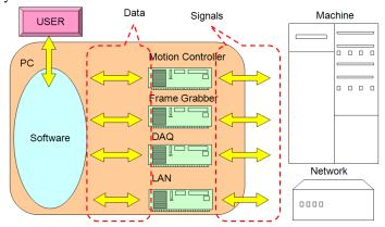
Figure 1. Interfacing concept of intelligent manufacturing machine
