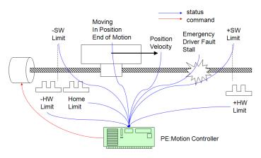
Figure 2. General function of motion controller
