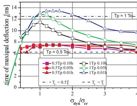
**Figure 7** Influence of pulse duration on time of maximal deflection appearance (cubic column of equal wall thickness, rectangular pulse)
