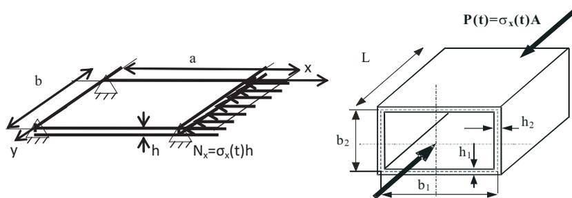
Figure 1 Simply supported plate and thin-walled column ( $A$  – cross-section area)
