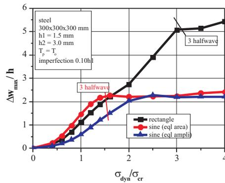
**Figure 5** Influence of pulse shape on column dynamic response (cubic column of different wall thickness)
