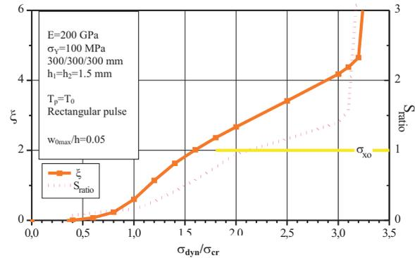
**Figure 8** Dimensionless maximal dynamic deflection  $\xi = \Delta w_{max}/h$  and effective stress ratio for cubic column (material characteristic)
