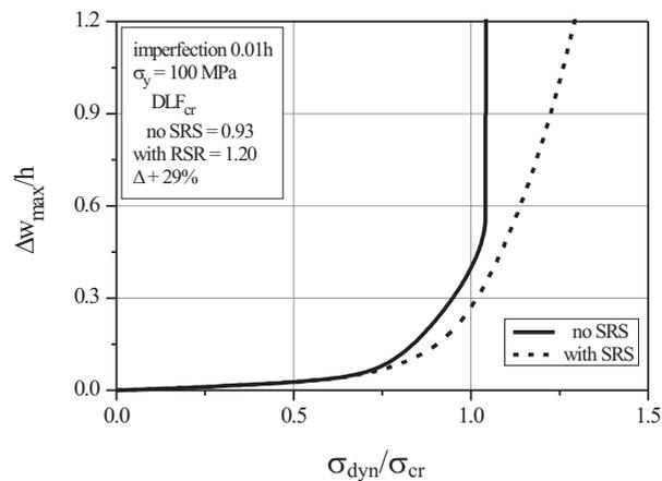
**Figure 9** Maximal column deflections versus dynamic load (rectangular pulse) (strain rate effect included)
