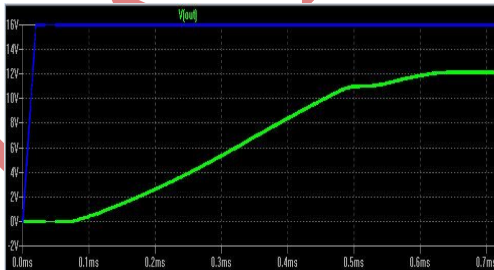
Figure 4. Simulation of (Buck- Boost converter) at Buck state
