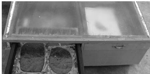
Fig. 2. Mango pulp drying in prototype solar dryer.
