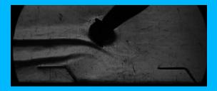
Fig. 12(a). Streamlines for the vertical oriented EHD ESP using the Schlieren photograph for vertically oriented EHD ESP
