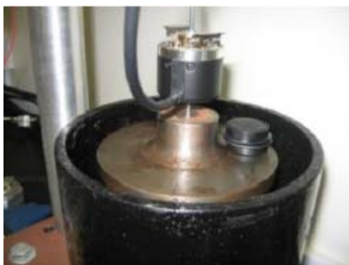
Figure 1. Laboratory set-up with unbalanced drill bit.
