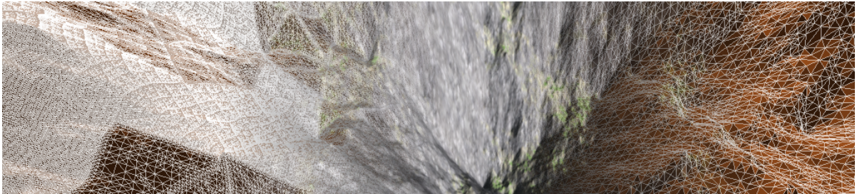
Figure 7: Comparison of preprocessed and dynamic triangulation of patches. left: static pre-generated patch triangulation; middle: textured representation; right: dynamic triangulation generated by our hybrid approach. Notice the significant reduction of triangle count on the right side.
