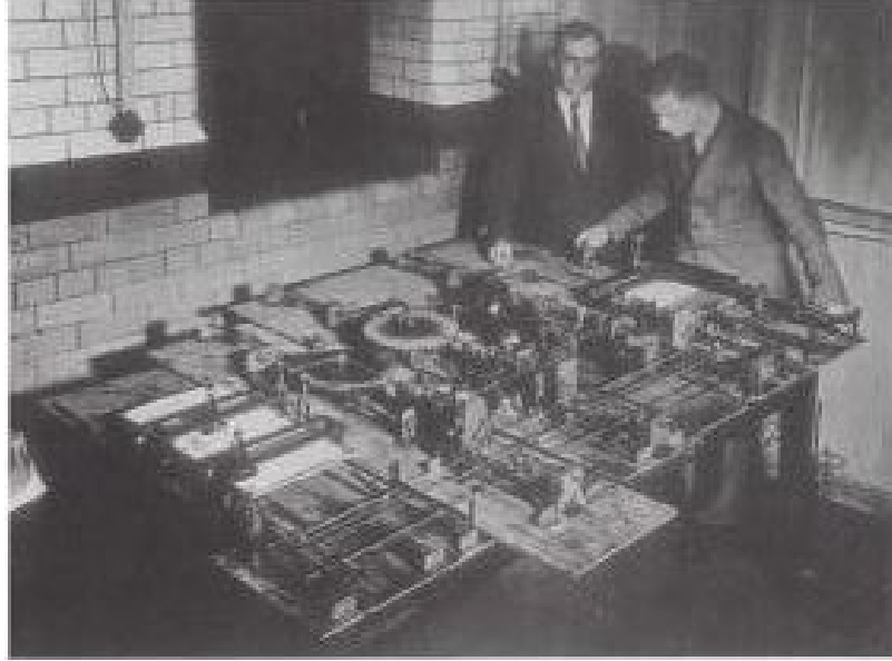
Figure 1.1: Dr. Douglas Hartree and Dr. Arthur Porter working on their differential analyzer.
