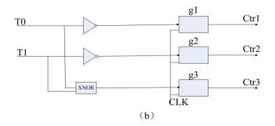
Fig.4. (a) A gated distributed BIST structure with encoder (b) Encoder and gating circuit
