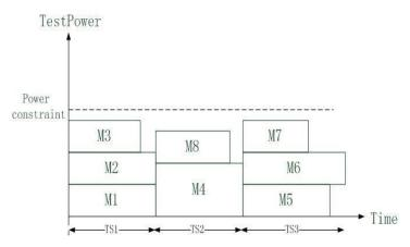
Fig. 1 . An example of test grouping results of 8 memories
