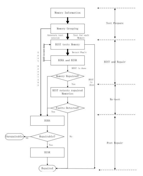
Fig.2. A revised memory test flow
