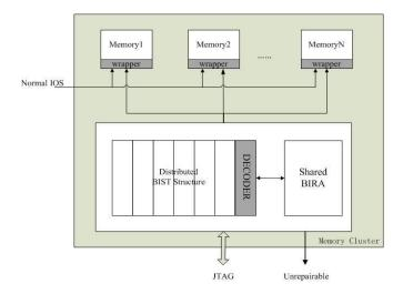
Fig.3. Overall framework of a dedicated test design
