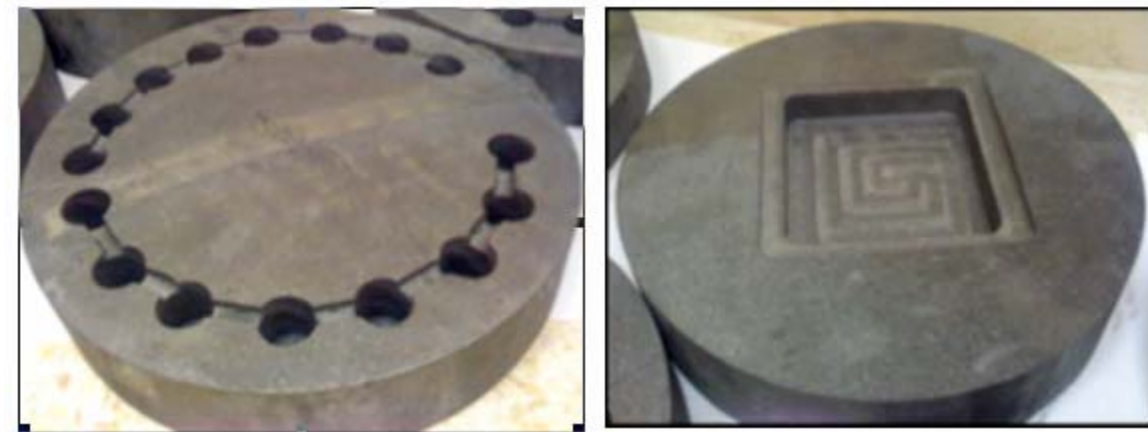
Figure 2 Graphite dies (a) cylindrical specimens and (b) flat plate specimens
