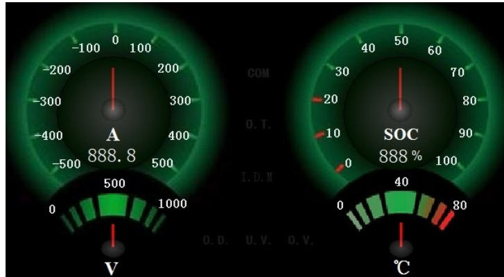
Figure 4: Monitoring SOC, drawn current using gauge diagram
