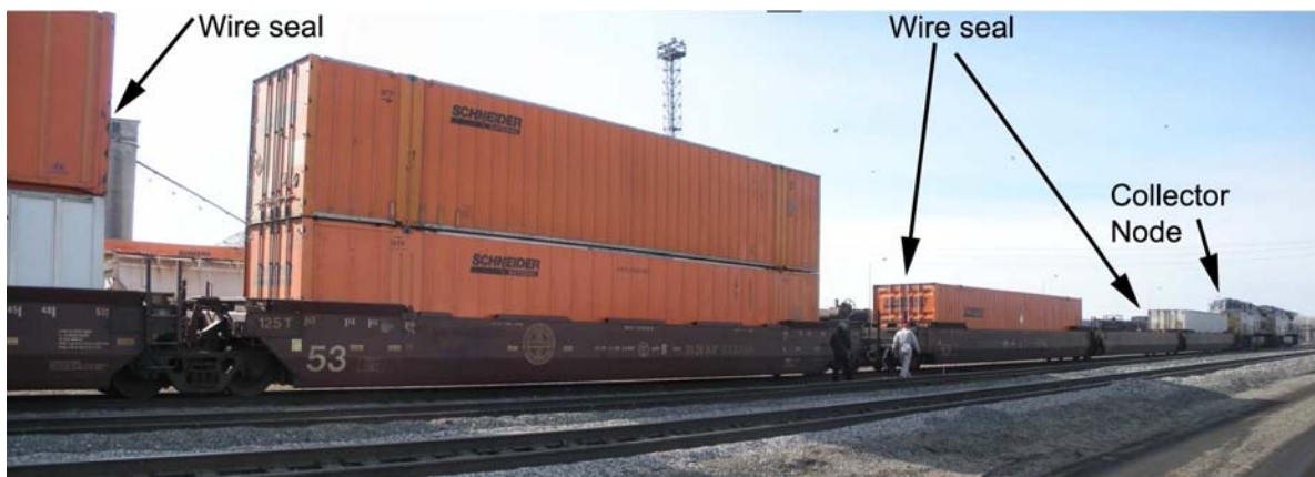
Fig. 8. Collector Node and Sensor Deployment During Short-haul Rail Trial
