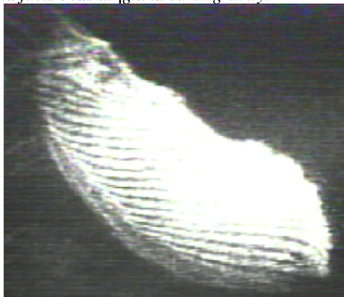
Figure 8. Image of Interferometer from the side of the fuel, and the upper black region represent the thick volume of the flame. (a) Microgravity
