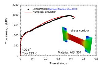
Figure 1. Comparison between numerical predictions of the **FE** model and experiments at 100 s<sup>-1</sup> and  $T_0=293$  K [6].
