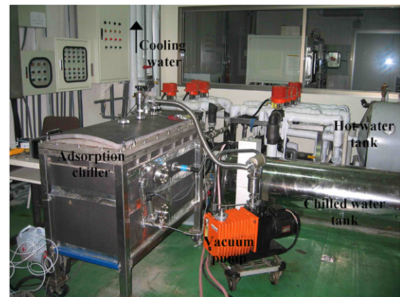
Fig. 3. Photograph of experimental facility.
