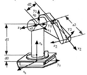
Figure 2: A PUMA 550 Manipulator Mounted on a Six-Axis Force/Torque Sensor.
