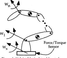
Figure 1: N-Joint Manipulator Mounted on a Force/Torque Sensor
